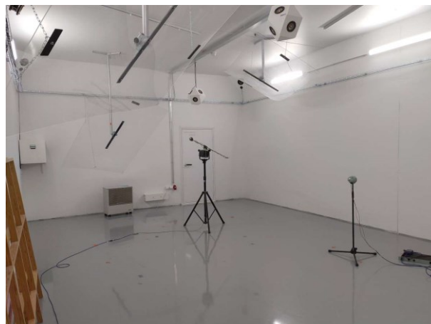
Figure A3.3. The reverberation room without the test specimen.
