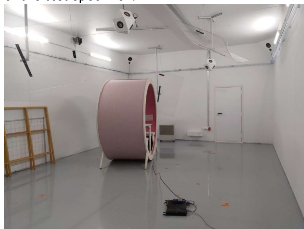
Figure A3.2. The test specimen in the measurement location in the reverberation room.
