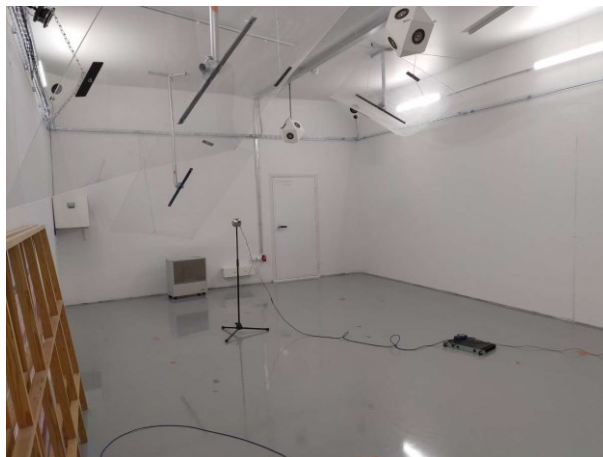
Figure A3.2. The sound source in position 2 in the empty reverberation room without test specimen.
